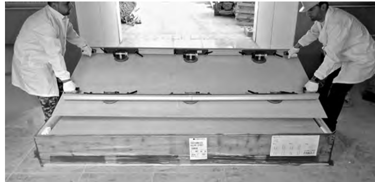
Aluminium frame with suction cups – this system is convenient because it can be dismantled for transportation purposes
